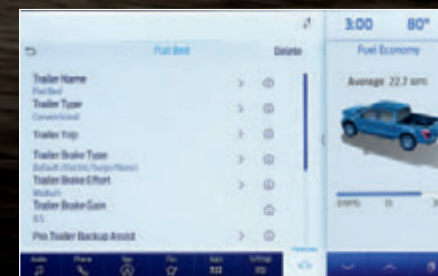
SIMPLE TRAILER SETUP A Quick Start Guide helps program trailers into available Pro Trailer Backup Assist.
