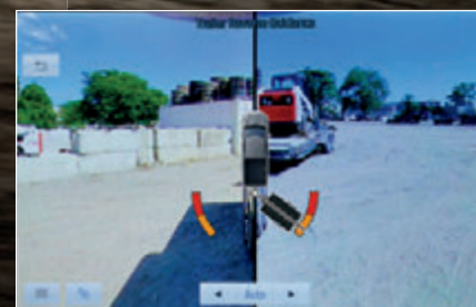
NEW TRAILER REVERSE GUIDANCE Available feature provides camera views and graphics to help you back up and park a trailer.
