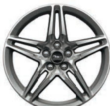
19" x 9" front/19" x 9.5" rear Luster Nickel-Painted Forged Aluminum 3 [Optional LHD/RHD]
